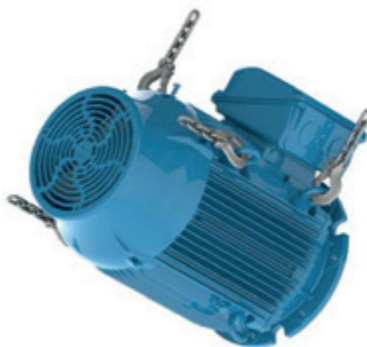
Figure 4.18 - Motor is being rotated to horizontal position
