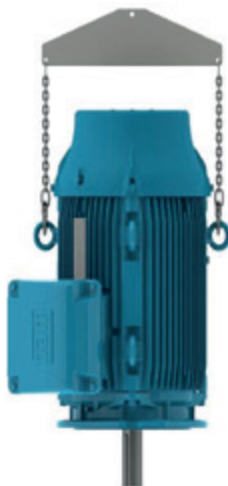
Figure 4.7 - Lifting of vertical mounted motors
