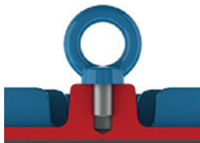
Figure 4.1 - Correct tightening of the eyebolt
