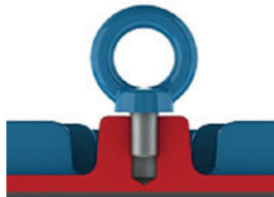
Figure 4.2 - Incorrect tightening of the eyebolt
