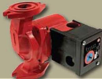
NRF-VS Pump Control is a versatile variable speed control for use in hydronic heating and cooling applications. Water temperature is controlled by regulating the speed of the pump which injects water from a different temperature water loop into a controlled loop.
