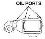
**NOTE:** The position of the conduit box is determined by the model of the motor used. The oiling ports must always be in the up position.
