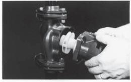
Loosen the four body cap screws. Shift the bearing assembly position slightly to allow for any pressurized water to escape.
