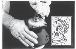
Remove the Impeller Nut and Impeller. Important: Note the following before installing impeller on new bearing assembly. If impeller is metal with flat back as illustrated in insert, the brass metal washer must be used atop the seal spring. If the impeller has a shroud on the back, DO NOT USE THE BRASS WASHER.
