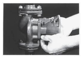
Fit the Bearing Assembly into the Pump Body and tighten Cap Screws evenly. Do not over tighten.
