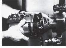
Use a box wrench to loosen the four motor cap screws and the motor is free from the bearing assembly.
