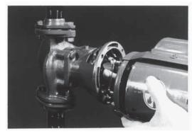
Connect the coupler to the Bearing Assembly Shaft and reposition motor.
