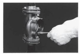
Replace the Body Gasket. The pump body should be cleaned of excess dirt and pieces of the old gasket.
